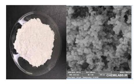
Hydrophobic silica is a form of silicon dioxide with hydrophobic groups chemically bonded to the surface. The hydrophobic groups are normally alkyl or polydimethylsiloxane chains.
