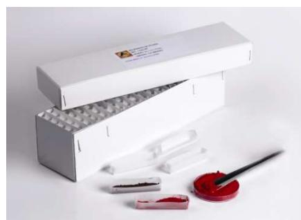
Small containers of parchment paper prepared for the weighing of viscous or pasty substances before the nitrogen determination by Kjeldahl method.
