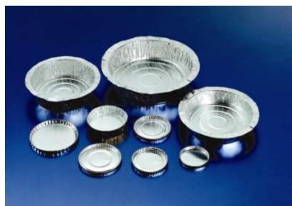
Practical trays for the weighing of all types of products in manual, electronic scales and dehydrators.
