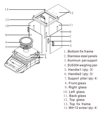
To install the glass windshield of balance, following parts in sequence:
